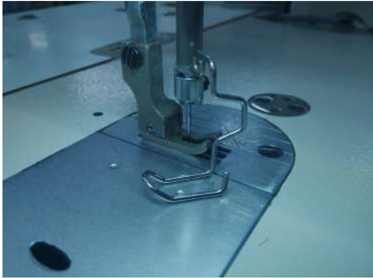
Picture 32: The presser foot, which is an equipment to protect fingers from getting injured, only installed when the auditors come.
