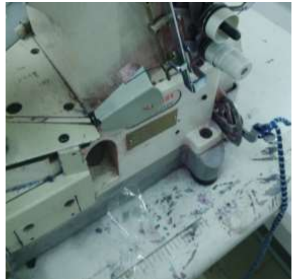
Picture 21, 22: Line Trimmers in Seduno and Cherry generates lots of floating dusts in the air.
