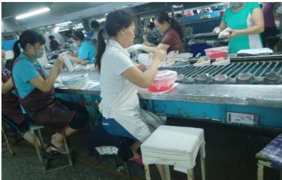
Picture 18: Some workers apply the glue on the shoes without wearing masks and gloves.
