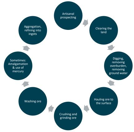
Prospecting, clearing the land from forest and shrubs, digging and removing the overburden until the mineralised layer or the ore is reached, pumping out groundwater, breaking the ore-bearing rock into smaller pieces and transporting the it to surface, crushing and grinding the ore into smaller pieces, transporting it to a water source and washing the ore to recover gold. From the first clearing of land to the first recovery of gold, up to 3-4 weeks may pass.<sup>34</sup>
